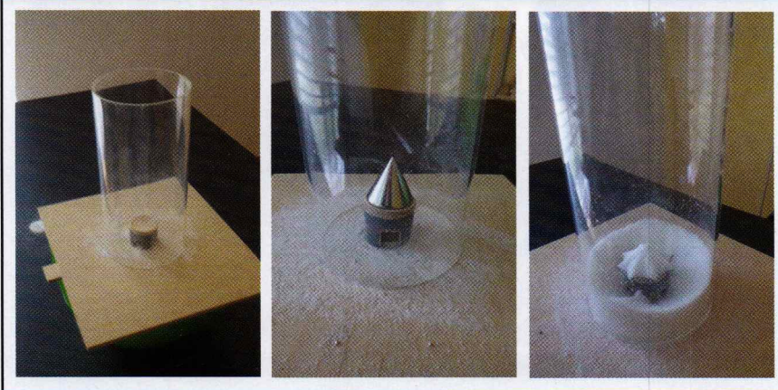
Figure 4: different shapes of silo tables were tested (L-R: round, cone, star shape) but were found to have little impact on the ease of discharge
